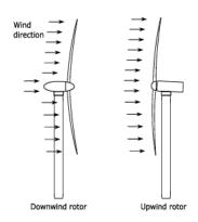
Figure A1: Diagram of downwind-rotor and upwind-rotor turbine desiges
