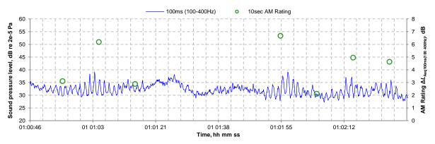
Figure 1: Amplitude modulation measured in wind turbine noise signal envelope
